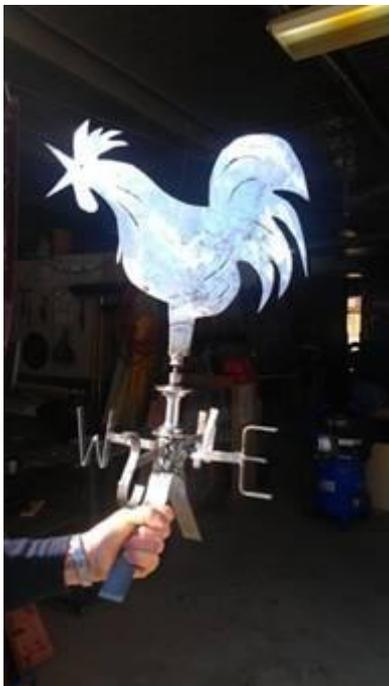
← Weathervane made by Al Phemister from mild steel (polished) – note the clever use of a bike wheel axle so the weathervane can swing with the breeze.
